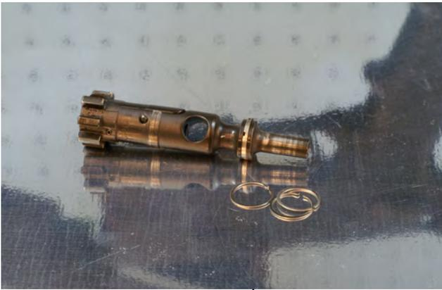
**Gas rings fail and also wear. They may or may not get to a failure stage before they have worn sufficiently to warrant replacement, and, hey, here's a good idea from that idea: just replace them every 1500 rounds. They're cheap and easy to change. Watch for cam pin wear. This part can get hammered shooting a lot of heavy loads. The bolt stop gets almost continual use by the High Power shooter who's single-loading the majority of his rounds.**
