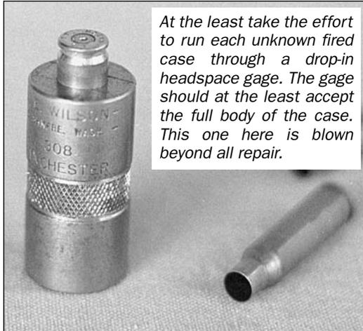
At the least take the effort to run each unknown fired case through a drop-in headspace gage. The gage should at the least accept the full body of the case. This one here is blown beyond all repair.
