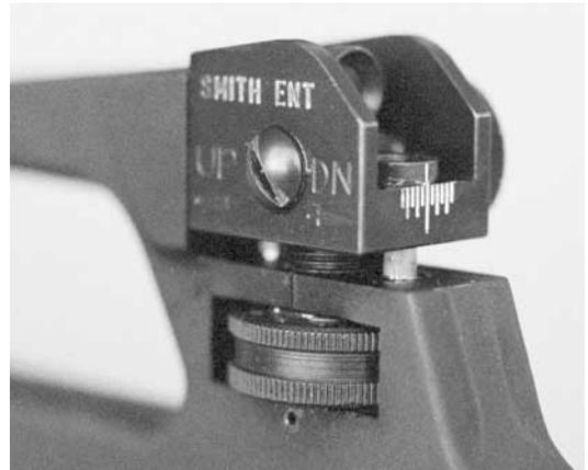
1. Extra detent added to elevation wheel for equal support.
