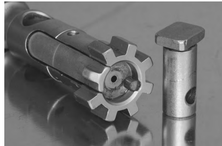
Well less worn. Here's a Smith Ent. chrome bolt and cam pin after about the same number of rounds. The bolt took a few hits from primer problems and the coating does protect the steel underneath from much routine wear. Good chrome is very hard.
