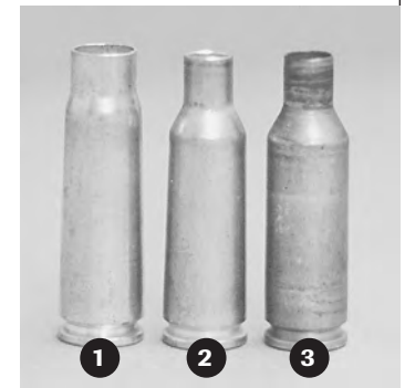
Want more? Just get it. Here's a .22 PPC next to a "tall-boy" version, resulting from additional room given in the chamber when the barrel was chambered. That's easy. There's about another grain propellant capacity. I think this sort of approach should be taken only with self-made cases from 7.62x39mm parent brass. That's because they have additional "material," in a way of looking at it, to endure the expansion and resultant larger final dimensions than starting with a PPC parent case. They are stronger than catalog PPC cases.
