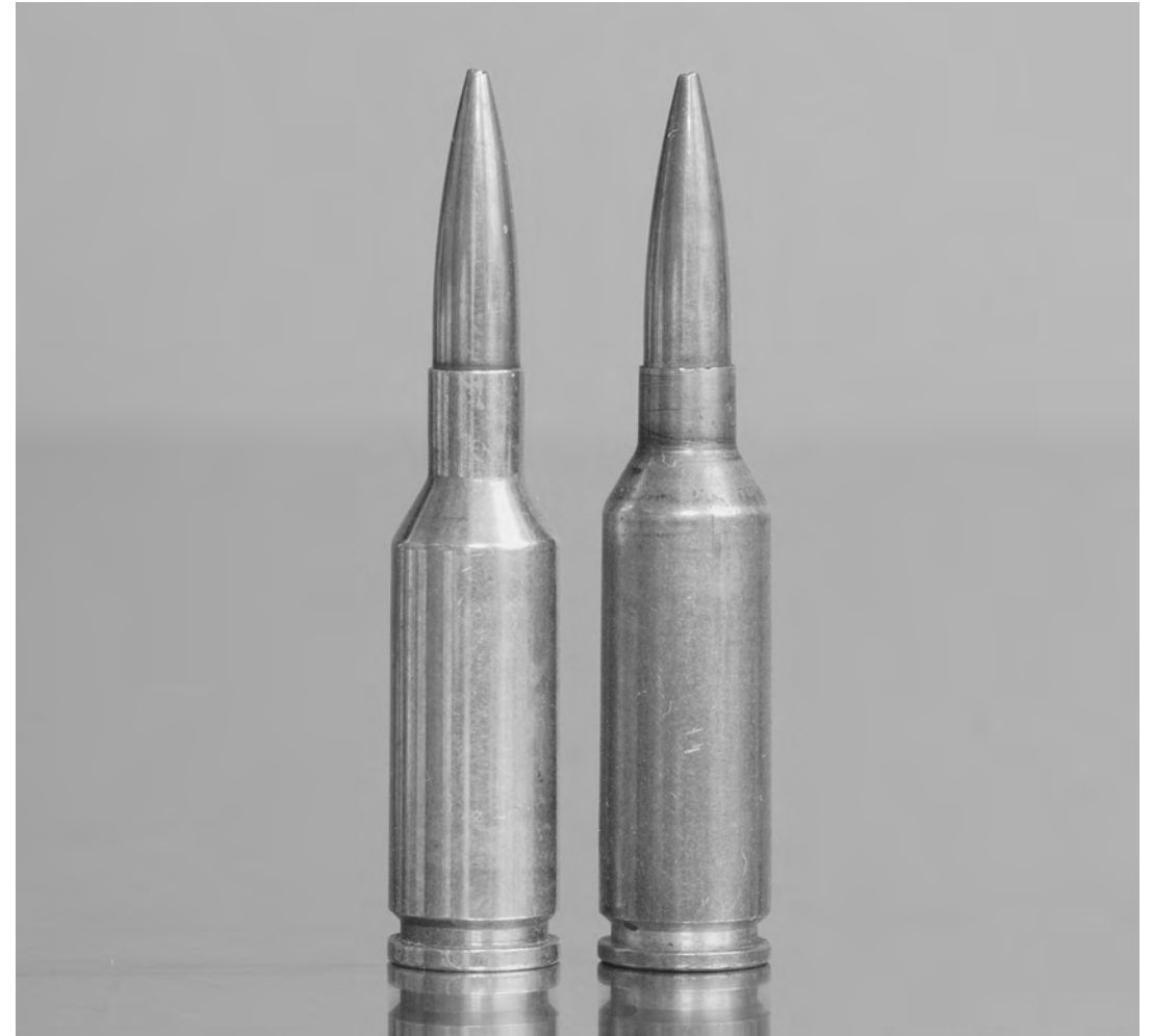
Want more? Just get it. Here's a .22 PPC next to a "tall-boy" version, resulting from additional room given in the chamber when the barrel was chambered. That's easy. There's about another grain propellant capacity. I think this sort of approach should be taken only with self-made cases from 7.62x39mm parent brass. That's because they have additional "material," in a way of looking at it, to endure the expansion and resultant larger final dimensions than starting with a PPC parent case. They are stronger than catalog PPC cases.
