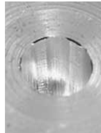
Polygonal rifling looks like a stretched "M" with no sharp lines. There is no sharp trailing or leading edge angles. In a conventionally rifled barrel, the leading and trailing edges of the rifling never obturates or fully fits that groove so, consequently, there is some gas blowby. How well a bullet conforms to the bore, and how little deformation or stress is on it has to make a difference. Better fit contact and more even bearing means there should be less displacement of jacket material.
