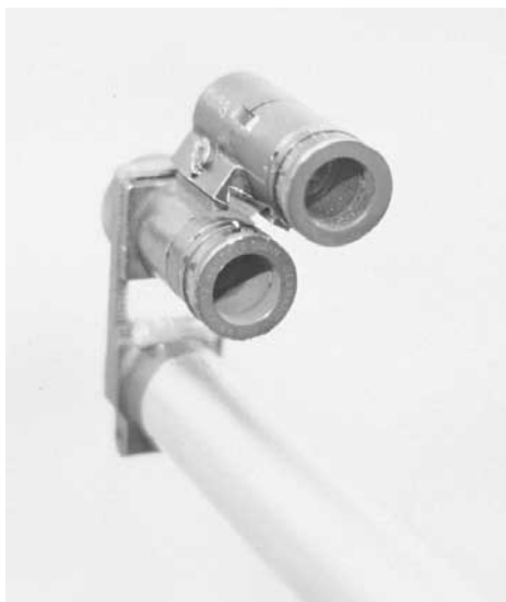
Here is the set up I used for a time on my Model 70. This sight dovetail was offset to level it to the cant I used offhand and also elevated. The idea to add another dovetail to the existing front globe used for sling supported positions was to get the sighting plane higher. That then allowed me to attain a better offhand position since it influenced several major technical areas in my hold. I used a separate rear sight. This sight was mounted on a taller rear sight base that was also ground to level the rear sight to the extra cant. I installed the sight and base prior to shooting offhand and then removed it to install the sight and base I used for the other events.
